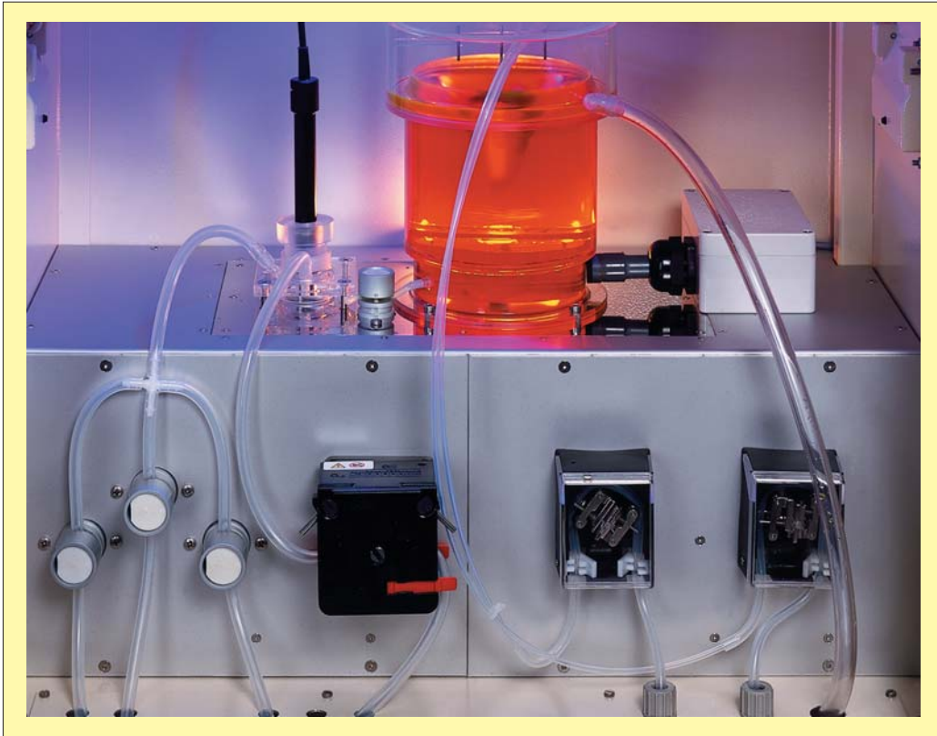
Fig. 3: Inside the NitritoxMonitor
